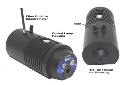
BIP2.0 is a compact, fiber coupled integrating sphere device designed as a sampling accessory for measuring diffuse reflectance using any fiber optic spectrometer from B&W Tek, Inc. The two inch diameter integrating sphere is machined from PTFE which is highly reflective (>97%) over a broad spectral range of 350 to > 2600nm.
